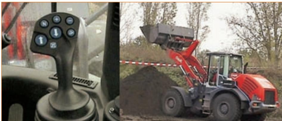
*Multi-purpose control joysticks in earth-moving machinery
