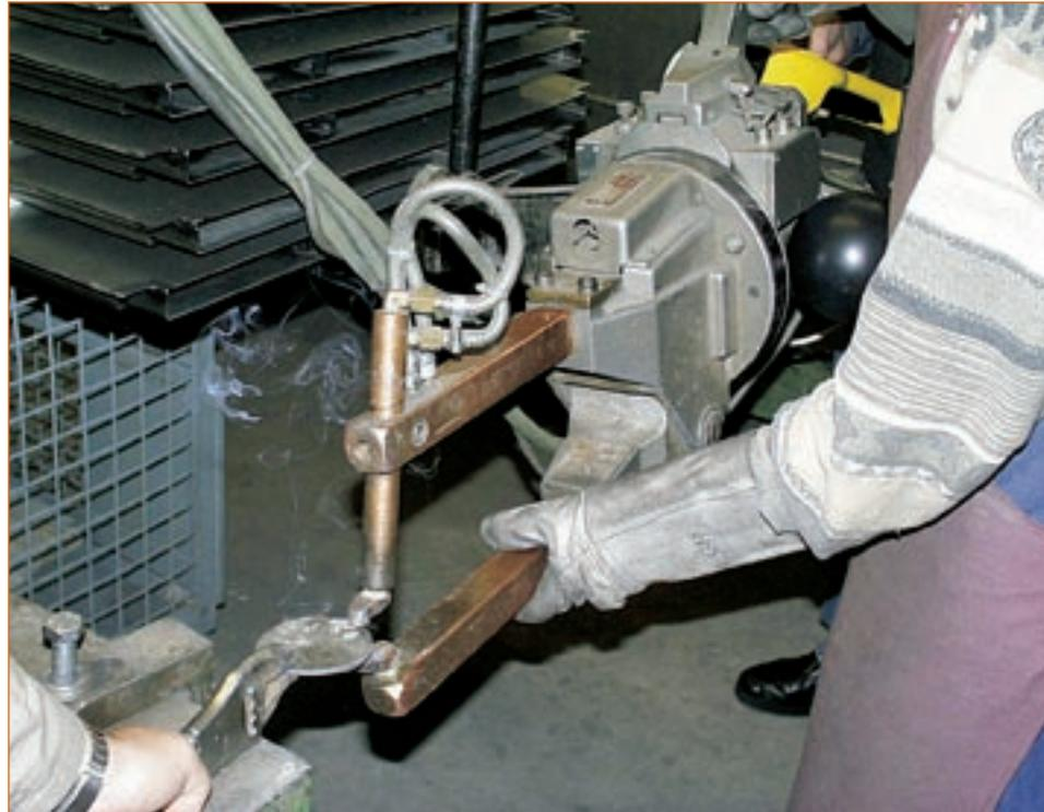
Emission of electromagnetic fields by a spot-welding gun
